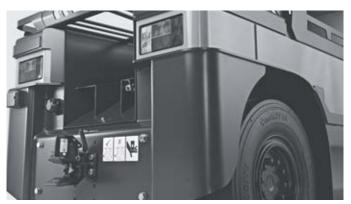
R 07 electric tractor: trailer coupling for use as a towing vehicle
