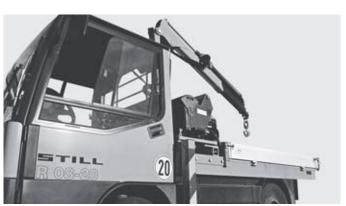
Optional built-in crane for lifting heavy loads
