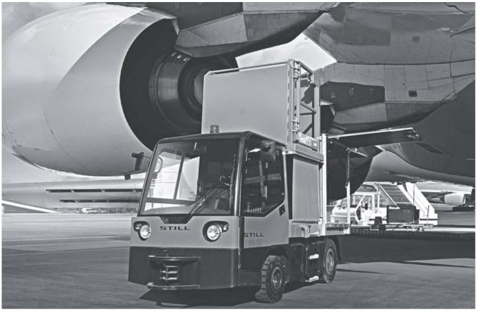
R 08 electric platform truck with optional aerial work platform and assembly platform
