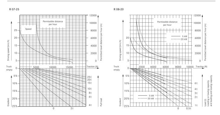
The speed and traction of the tractor can be programmed within the two curves in order to achieve the desired application. The permitted travel distance per hour is the total distance including return journeys and downhill sections (descents). The use of braked trailers is recommended if trailer weight exceeds 9 tonnes or downhill sections are to be traversed.
